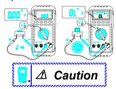
For in-circuit test, turns circuit power off and Discharge the high-voltage capacitors through an appropriate resistance load.
