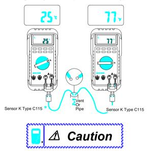
Do not Connect senor K Type C115 (Bead probe) to live Circuits.
