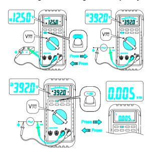
Note – When measuring voltage, the Meter acts like a  $10M\Omega$  impedance in parallel with the circuit under test. This loading effect of the  $10M\Omega$  of the Meter can cause measurement errors, *loading effect error*, Especially in high impedance circuits.
