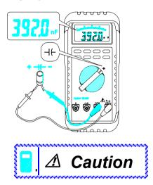
To avoid possible damage to the meter or to the equipment under test, disconnect circuit power and discharge all high-voltage capacitors before measuring capacitance. Use the DC voltage function to confirm that the capacitor discharged.
